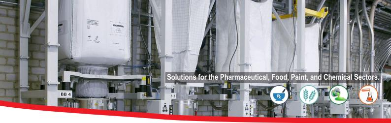
ProChem's big bag filling machines have been designed to fill even the most difficult to handle materials, using a time proven technique which involves high precision weighing coupled with a truncated pyramid table with vibrators, the filled material is weighed deaerated and densified before leaving the filling station. The ultimate
